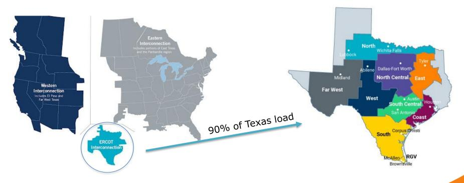
ERCOT is composed of the interconnected network of highvoltage transmission lines & power plants in the region.
